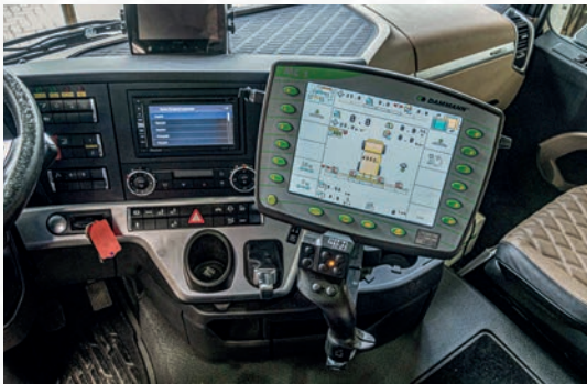
(Abb. 5: Terminal MC1 / Fig. 5: Terminal MC 1)
