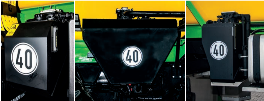
Abb. 20. Hydraulik-Tanks: DT2800H/DT3500H/DT2400H Highlander
